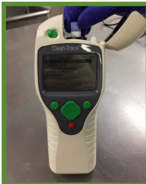
Figure 2. Placing an ATP swab in the luminometer for measurement.
